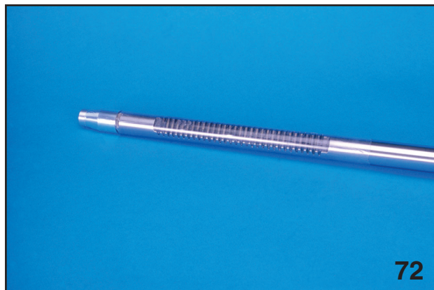
Rack Cover Installed
