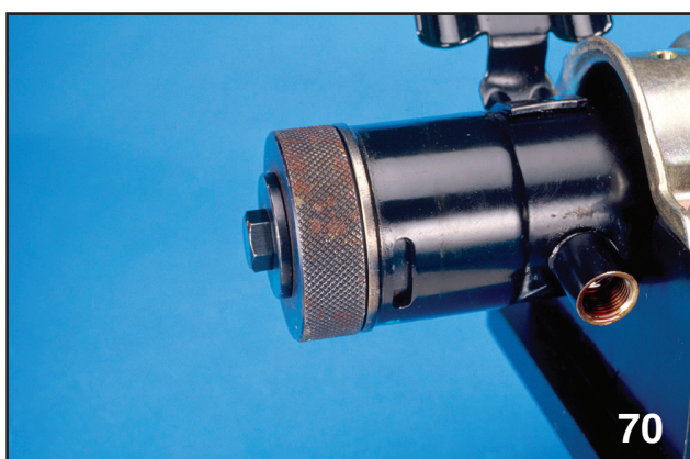
Inner Seal Installed
